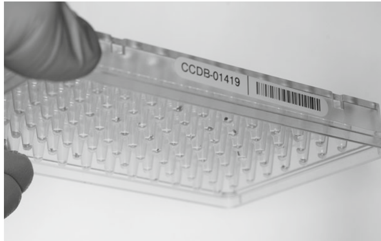
Fig. 1. 96-Well microplate shown from below demonstrating the recommended amount of tissue to sample in each well.
