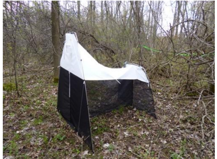
Figure 1. Malaise trap deployed at Boyne Valley Provincial Park in 2014.
