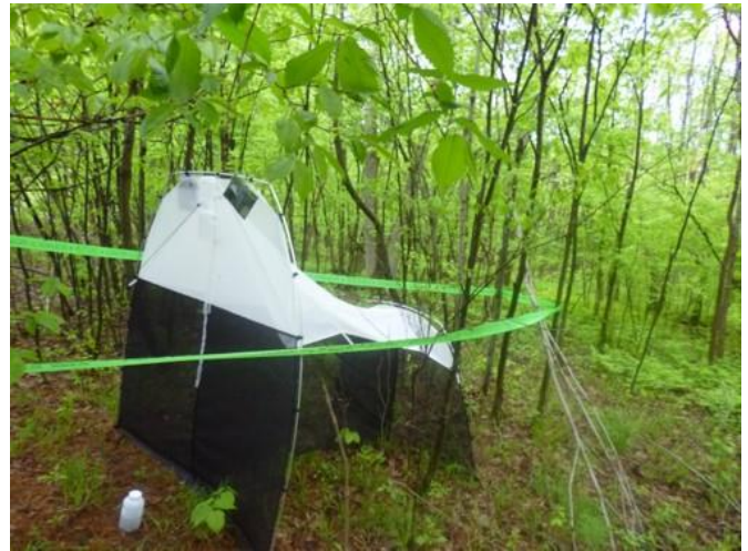
Figure 1. Malaise trap deployed at the Charleston Lake Provincial Park in 2014.
