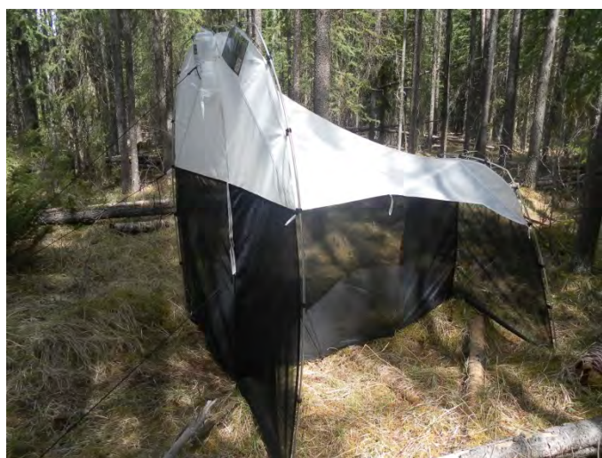
Figure 15. Malaise trap deployed at Kootenay National Park in 2014.
