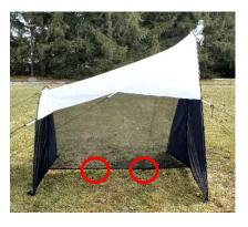
10. Attach the guy lines to the trap and adjust them so that the trap erects in a proper shape and tension. Peg the guy lines into the ground using pins and stakes. Alternatively, tie the front and/or back lines to nearby trees for added support when possible.
