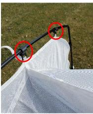
8. With two people, stand up both mesh panels temporarily from the top of the poles to erect the trap. The inverted Y-shaped collection head should sit over top of the long pole. Please double check that the moth excluder at the trap head has been removed; in case it is still on, please take it out by pushing and twisting it through the trap head.
